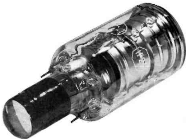
FIG. 1. IMAGE TUBE—This is the RCA 1P25 image tube used in infrared viewing devices. The image tube, an RCA development, transforms an invisible (infrared) scene focused on the large end of the tube into a visible picture on the small end.
