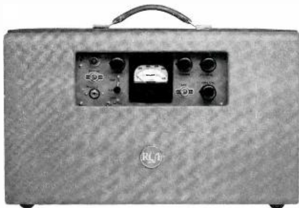
FIG. 18. The receiver control unit includes additional i-f stages, two limiter-discriminator channels, a video amplifier, and monitoring circuits.
