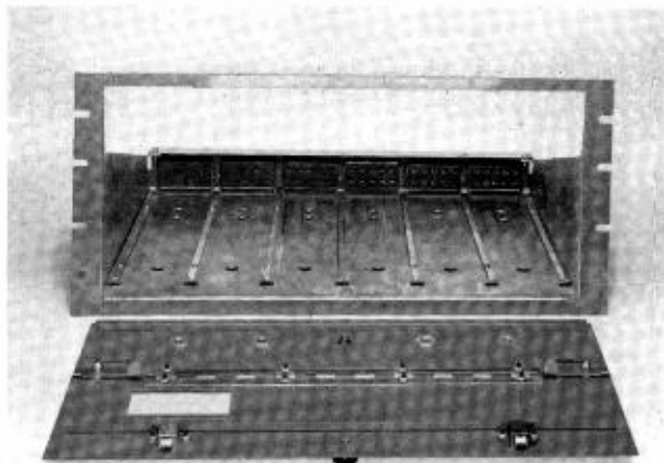
FIG. 5. Center section of RR-2A front panel is held in place by snap fasteners—can be easily removed.
