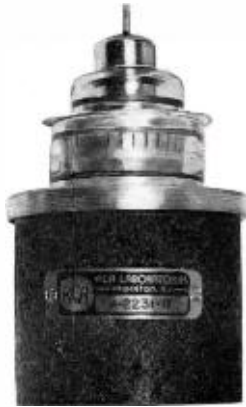
FIG. 9. 500,000 WATTS —That's what the RCA Type A-2231 Pulse Triodes put out (pulsed service) at 600 mc! This tube, shown above, was developed for high-power radar applications.
