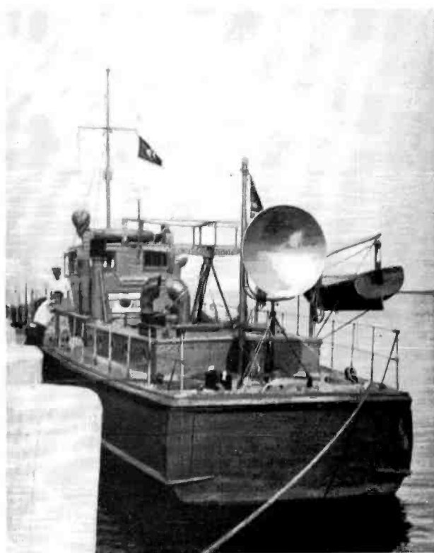
FIG. 5. This view shows the 9 cm. receiver (used with the transmitter shown above) installed on an army boat in New York harbor.
