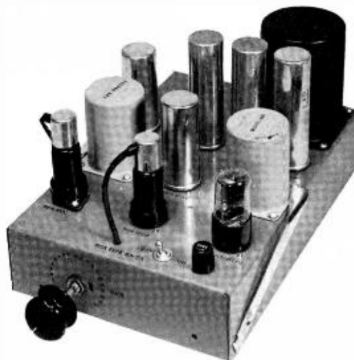
FIG. 13. Type BA-2A Booster Amplifier is a two-stage with self-contained power supply, low noise level and gain of 50 db.
