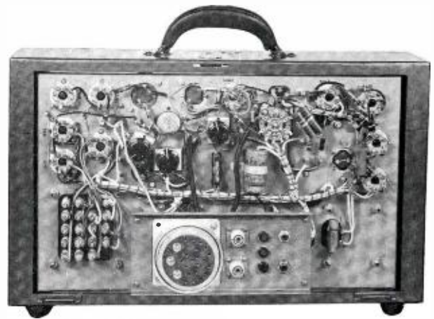
FIG. 14. Rear of the transmitter control unit. Front and rear covers are of the snap-on type, easily removed.
