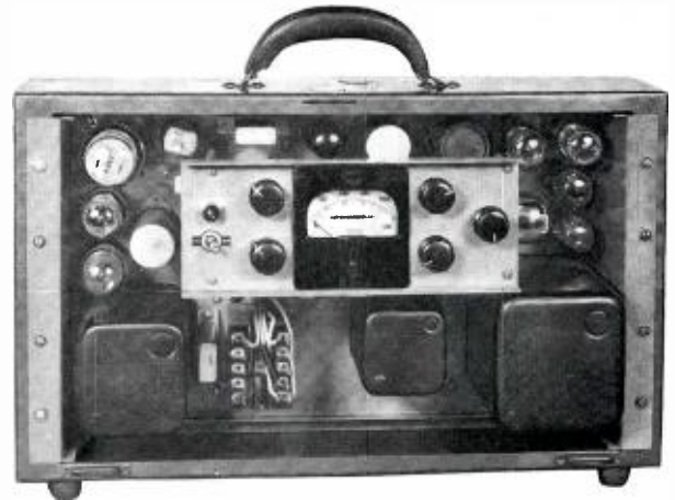
FIG. 13. Interior of the transmitter control unit. All components are mounted on a standard bathtub-type chassis, which can be mounted on a relay rack or in a suitcase-type carrying case as shown here.
