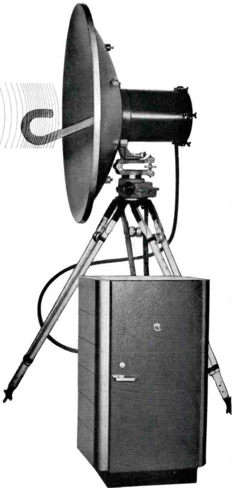
FIG. 2. This is the microwave receiving equipment. It consists of a parabolic antenna (identical to that at the transmitter), the receiver pre-amplifier, (in the cylindrical case attached to the rear of the parabola), the receiver control unit, and a power supply unit. The last two are mounted in the cabinet at the bottom. The control unit in a portable case is shown in Fig. 17.
