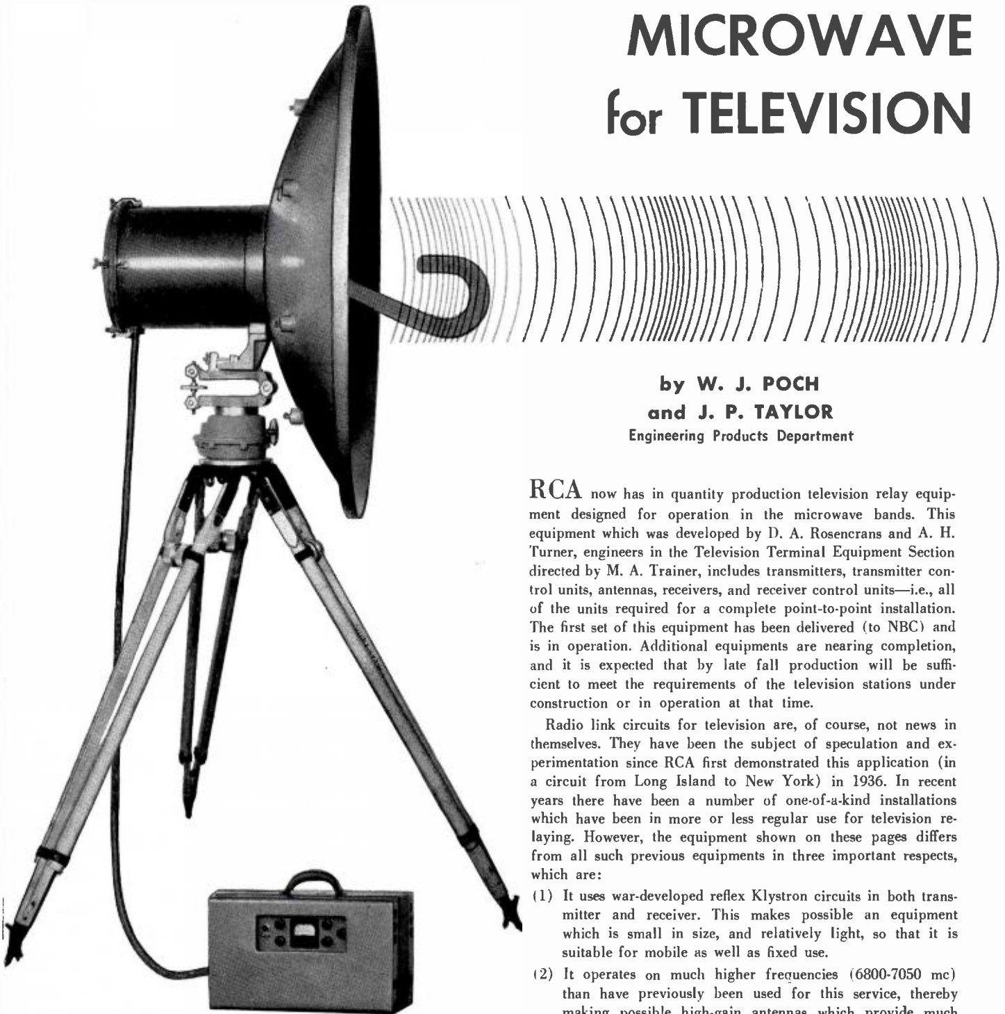
FIG. 1. This is the complete microwave transmitting equipment. It consists of the parabolic antenna, the transmitter proper, (in the case attached to the rear of the parabola), and the transmitter control unit. This antenna has a power "gain" of 5000 (which gives an "equivalent power" of 500 watts with a transmitter output of only 100 milliwatts).
