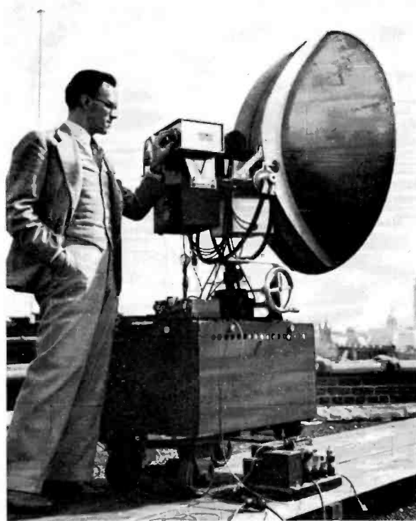
FIG. 6. This view shows Dr. Linder with a 9 cm. pulse transmitter located on the roof of an RCA building in Camden in 1936.
