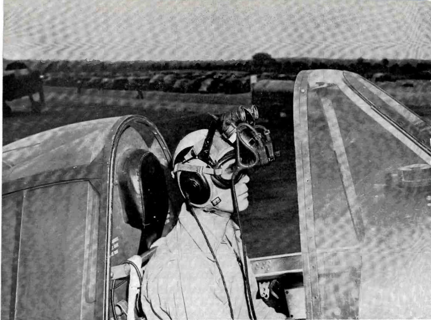
INFRARED FLYING HELMET—For night flying provided the best means of identifying and following enemy planes at close range.
